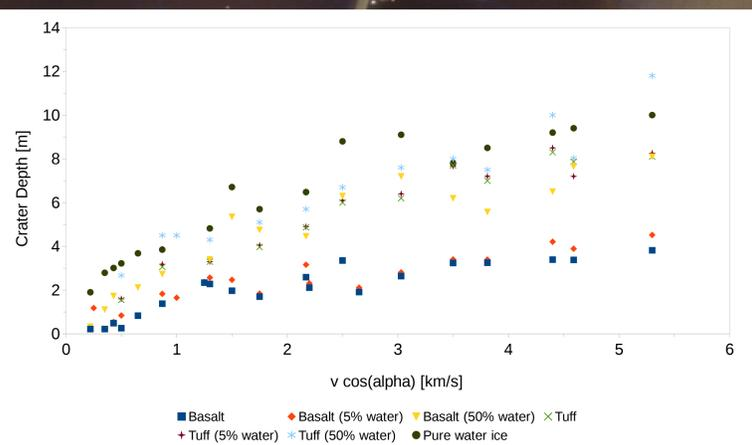
**Figure 3.** Variations of crater depth in terms of the vertical component of the impact velocity for different target materials. The craters are up to about 12 meters deep.
