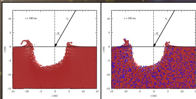
**Figure 2.** Craters resulting from the same projectile as in Fig. 1 hitting a softer tuff target with water-ice fractions of 0 wt-% (left) and 5 wt-% (right). The resulting crater depths are 7.0 m and 7.2 m, respectively.
