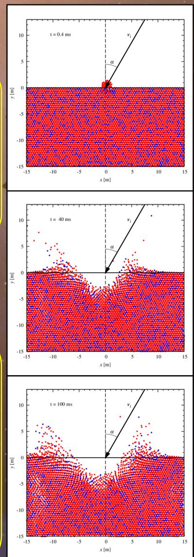
**Figure 1.** Snapshots of an impact at 4.4 km/s and a 30° angle. The target has 5 wt-% water ice (blue dots), the resulting crater depth is approx. 3.4 m.
