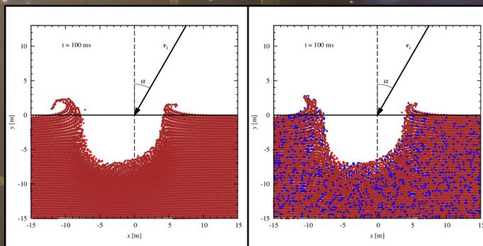
**Figure 2.** Craters resulting from the same projectile as in Fig. 1 hitting a softer tuff target with water-ice fractions of 0 wt-% (left) and 5 wt-% (right). The resulting crater depths are 7.0 m and 7.2 m, respectively.
